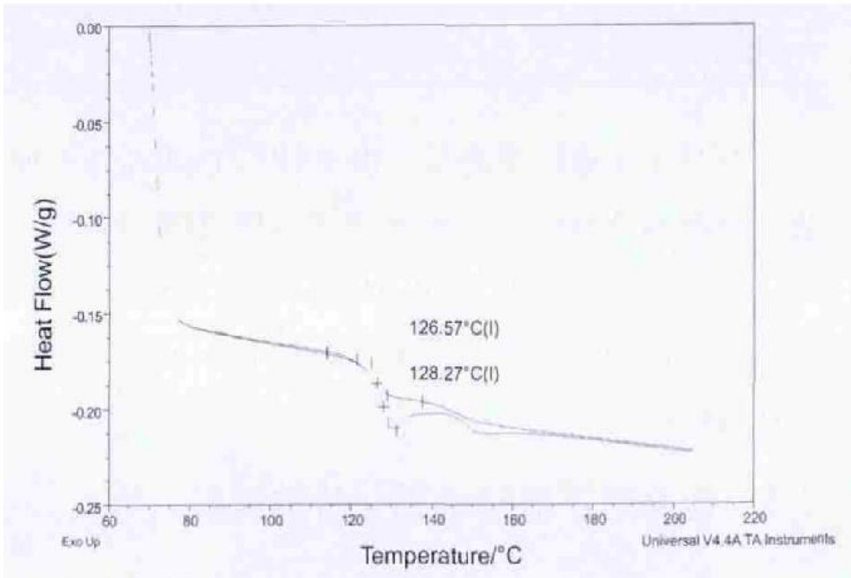
Fig.5 SP120N Tg test curve
