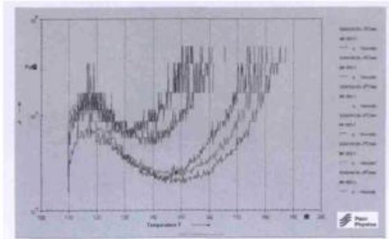
**Fig 4 the resin melt viscosity curve in different heating rate**
