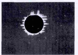
Fig. 8 Ordinary FR4 material (1080 prepreg) hole wall quality
